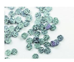
Up until 2014, osmium was available only in its powdery, toxic raw form. Due to its rarity and toxicity, raw osmium had few scientific uses, and even fewer industrial applications. Only when Swiss scientists discovered the process required to crystallize the raw form into solid bars was osmium able to be handled safely.
